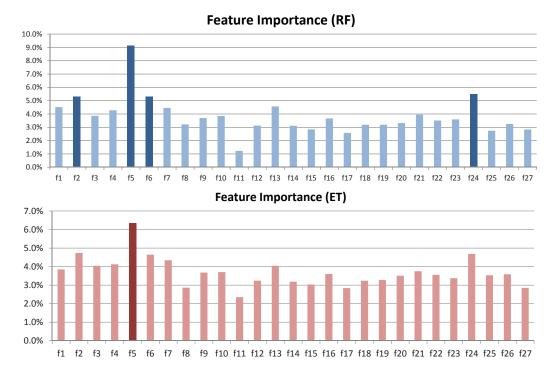
**Figure 7:** The importance of the 27 proposed features for the classification of the emotions; features with more than 5% weight of impact are highlighted. The upper diagram shows the importance of the features when Random Forests (RF) were used, while the lower shows the importance for the case of Extremely Randomized Trees (ET).
