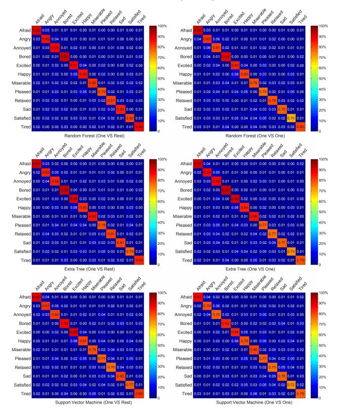
**Figure 6:** The confusion matrices of the emotion classification using six case scenarios. On the left side are the confusion matrices using the RF, ET and SVM classifiers, respectively, with the OvR strategy, whereas on the right side are the confusion matrices of the RF, ET and SVM classifiers using the OvO strategy.
